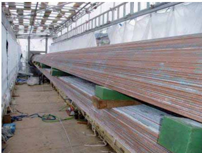
Internal inspection and broken wires (images: Engineer’s Journal - Engineers Ireland)
