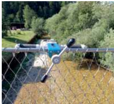
fig.: Tractel Dynarope, rope force measuring device
