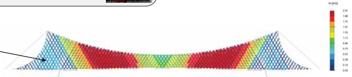
fig.: beam model, net i forces N [kN]; LC\{G + P + Q\}
